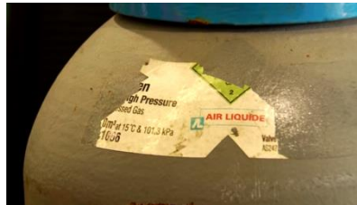
Avoid: Missing Label
